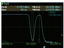
The falling signal edge shows an unwanted anomaly. The signal bounces back, after an initial decline, and then it settles to the actual off level.
