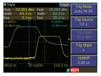
Both 4541 and 4542 power meters command powerful pulse recognition and analysis systems. Parameters like pulse-width, rise time, fall time, power distribution and many others are automatically detected, measured and presented.
